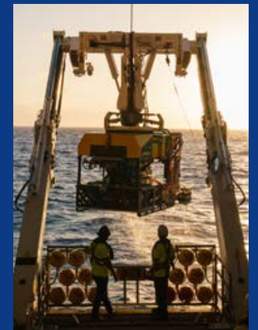
ROV deploys from Research Vessel Falkor (too) at the beginning of a scientific dive © Schmidt Ocean Institute
